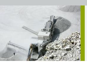
1 Fraunhofer expertise for sorting the heterogeneous building rubble in order to produce homogeneous construction products and secondary raw materials.
